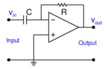
Interchanging the R and C in an integrator results in a differentiator.
