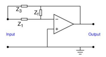
$$Z_f = Z_2 || R_2 = \frac{(1 + 2sR_1C)R_2}{1 + 2sR_1C + s^2R_1R_2C^2}$$
