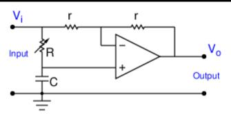
The voltage at the input pins is  $(V_i + V_o)/2$ . So
