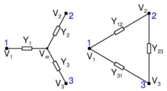
To derive the conditions, we first label the star and delta networks in terms of admittances. Here  $Y_1 = 1/Z_1$ ,  $Y_2 = 1/Z_2$ ,  $Y_3 = 1/Z_3$ ,  $Y_{23} = 1/Z_{23}$ ,  $Y_{31} = 1/Z_{31}$ , and  $Y_{12} = 1/Z_{12}$ . We have also indicated three arbitrary voltages  $V_1$ ,  $V_2$ , and  $V_3$ , at the three terminals. The voltage where the three star elements meet is indicated as  $V_m$ .  $V_m$  will be first be determined in terms of  $V_1$ ,  $V_2$ , and  $V_3$ .
