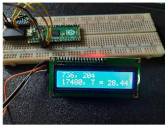
First line: *x* and *y* components of acceleration in device units Second line: *z* component of acceleration in device units, temperature Horizontal Board:  $a_z$ : 17480 device units
