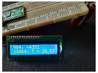
First line: *x* and *y* components of acceleration in device units Second line: *z* component of acceleration in device units, temperature Tilted Board:  $a_z$ : 16864 device units
