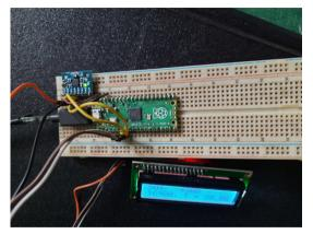
Small board: 16 mm  $\times$  20 mm, MPU6050 Accelerometer module ( $\approx$  Rs. 115) Big board: 22 mm  $\times$  53 mm, Raspberry Pi Pico Powered from the USB Port
