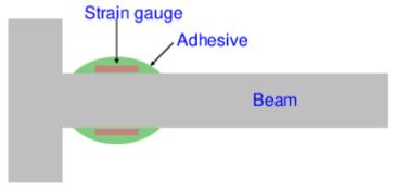
If the upper strain gauge is in the tension, the lower one will be in compression and vice versa.
