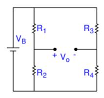
$$V_o = V_B \left( \frac{R_2}{R_1 + R_2} - \frac{R_4}{R_3 + R_4} \right)$$
