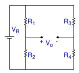
$$V_o = V_B \left( \frac{R_2}{R_1 + R_2} - \frac{R_4}{R_3 + R_4} \right) \tag{10}$$
