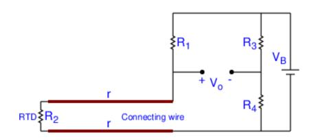
Disadvantage: r depends on the length of the connecting wire and only affects  $R_2$ .
