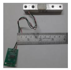
Note the white adhesive used to attach the strain gauge. The HX711 amplifier/digitizer board is also visible.
