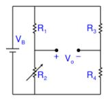
Advantage: No offset output. With minor adjustment, one can make the output nearly proportional to the input.
