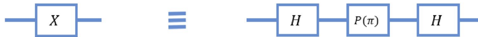
Figure 10. Schematic of quantum circuit for implementation of the Pauli X gate on a single qubit. This gate has a quantum time complexity of 3.
